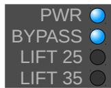
If you want to compare the corrected and uncorrected operation, press the BYPASS button quickly. This will switch between bypass and normal mode. The first press will set bypass mode, which is also indicated by the BYPASS LED being lit. If the Bypass mode is already active, the unit switches back to normal mode. In bypass mode no room corrections are active and user selected lifting EQ is turned off. Low-pass or dipole corrections remain active in bypass mode (Anti-Mode 8033S-II only).
