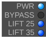
A fourth EQ setting activates the digital subsonic filter without any lift. The Subsonic-Filter-Only mode is active when the LIFT25 and LIFT35 LEDs are dimly lit. The “flat” setting is automatically changed to this setting after the first (main) calibration.
