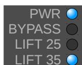
The third EQ setting is LIFT35. When LIFT35 LED is lit, Anti-Mode boosts frequencies between 25-35Hz (max. 8dB at 30Hz). As with LIFT25, the digital infrasonic filter is also activated.
